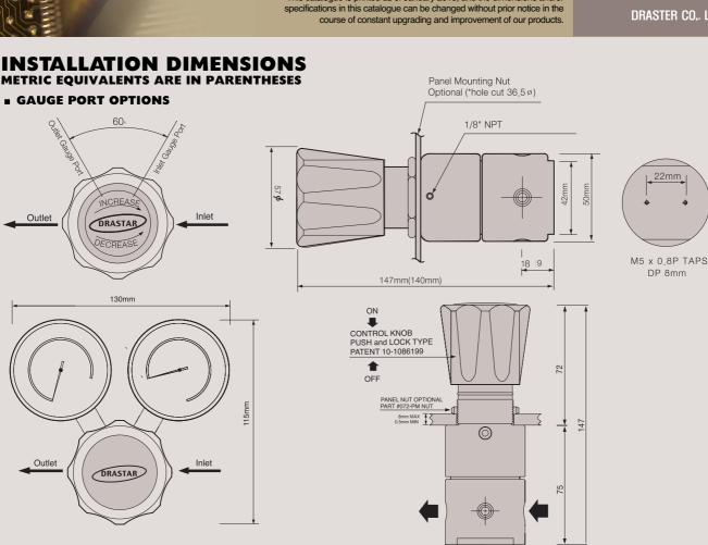
outside or minute vibration at the gas pipeline. You can prevent the self-changing of pre-set value just by pushing the handle and reset the value freely by drawing the handle. DRASTAR has created and applied patent for this push and lock system for DRASTAR regulators (patent number 10-1086199).
